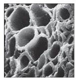
oxygen, carbon dioxide or other chemicals. In this manner the charcoal is broken down into even finer granules, thus creating a greater surface area and achieving an increased adsorptive capacity.
